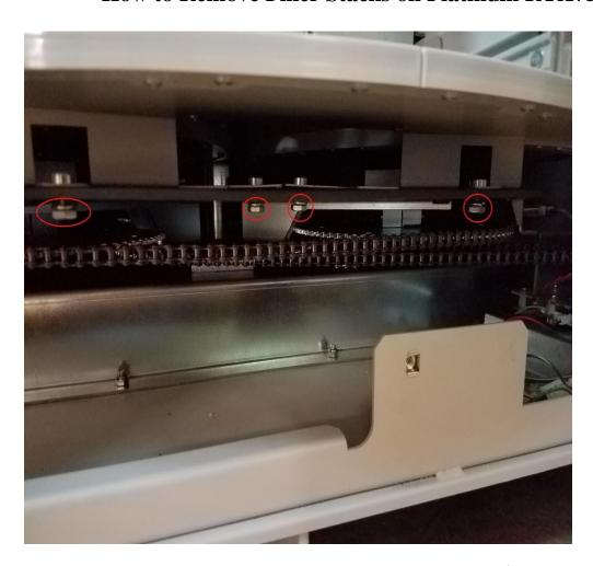
4. Use a step ladder to access the top of the filler stack. Using a  $7/16^{th}$  rotary ratchet remove the 3 bolts on top of the filler stack.
