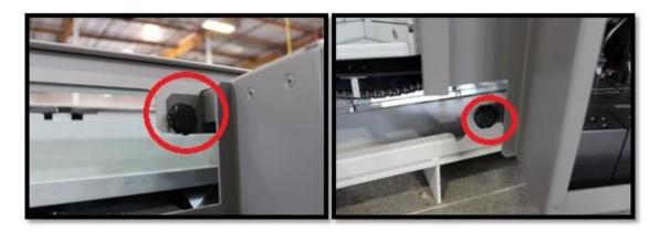
2. Rotate to filler stack near where you want to add/remove stack panels. It's preferable to remove a filler stack without a motor. (In our example we will be removing filler 101 which also houses 10A and 10B.)
